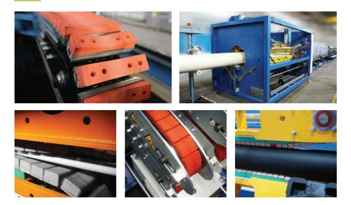
Take off pipes with 2, 3 or 4 tracks, with flat and shaped rubber pads, complete the lines. Special take off units with useful pick-up devices in length and width able to meet any special needs.
