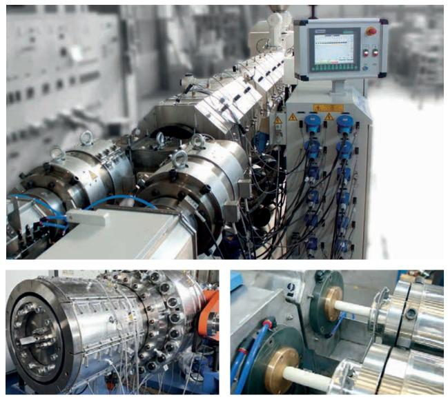
Each extrusion head is manufactured to meet the specific needs and process parameters of each processed material and desired final product.
