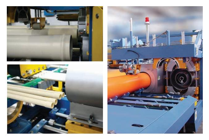
All our pipe production lines can be completed with the equipment required to widen and adapt the pipe inlets.
