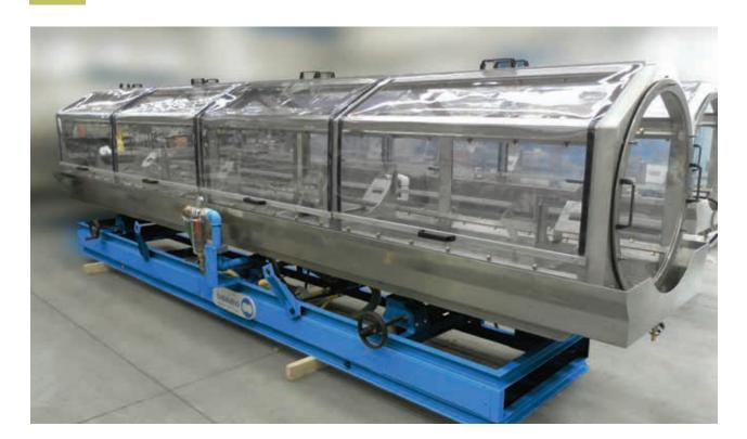
Designed for cooling of pipes with diameter up to 800 mm, it allows reaching high extruded material linear speeds, ensuring the maximum dimensional stability. The ease of adjustment on 3 axes and the motor-driven longitudinal movement allow quick and precise positioning during machining.
