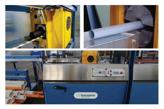
Modular and ergonomic unit, provided with automatic pneumatic movement that does not require manual operation for adjustments such as cut length, trolley forward and backward speed.
