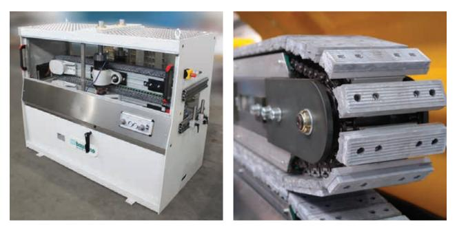
The take off units that complete the profile extrusion lines are sturdy and very reliable. Provided with track closure system with pneumatic regulation, they are available with special shape pads according to the type of extruded profile.
