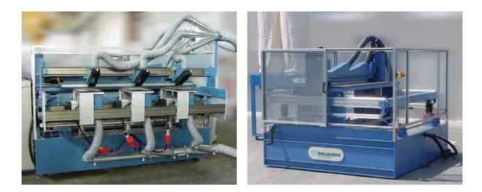
Longitudinal transfer horizontal cutters for profiles greater than 300 mm, provided with automatic pneumatic movement that does not require manual operator interventions, complete the profile lines.
