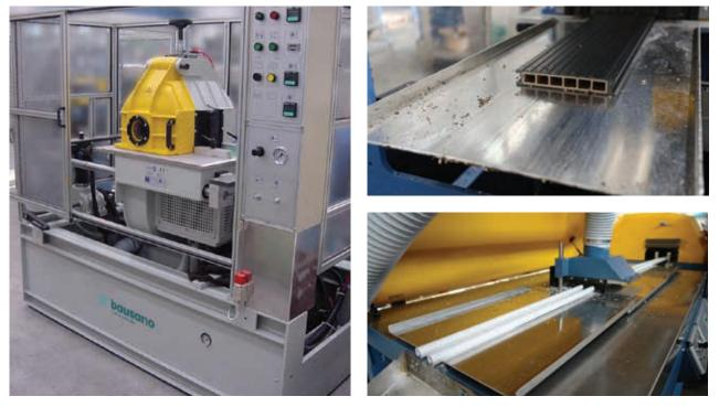
High cut speed vertical cutters for small profile complete the profile line.
